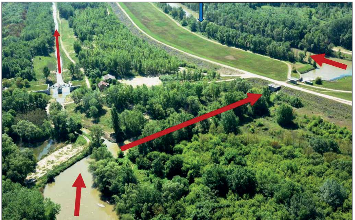
Figure 36: Flow in the supply channel and toe drain at the Rajka sluice gate
