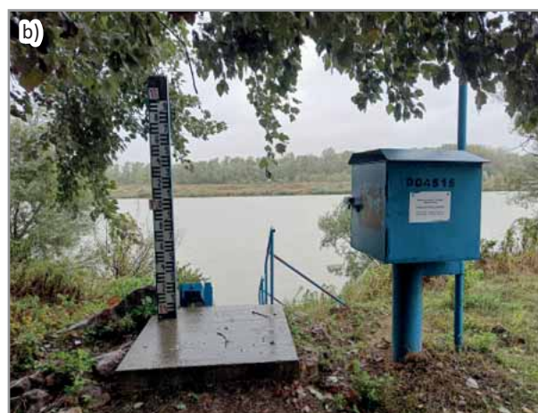
Figure 61: a) Locations of surface-water level gauging stations in Szigetköz. Gauging stations are monitoring points where river or channel water levels are measured regularly or continuously to track changes over time (Szűcs, 2009); b) Old Danube gauge at Doborgaz
