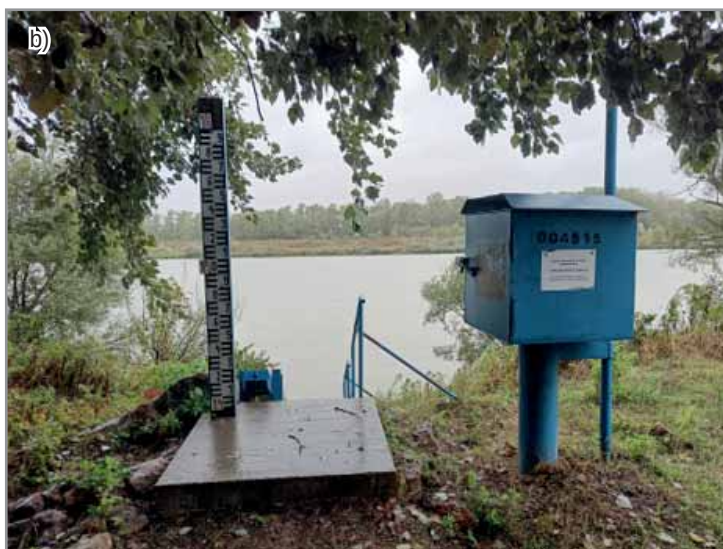
Figure 30: Locations of surface-water level gauging stations in Szigetköz. a) Gauging stations are monitoring points where river or channel water levels are measured regularly or continuously to track changes over time (Szűcs, 2018 ); b) Old Danube gauge at Doborgaz
